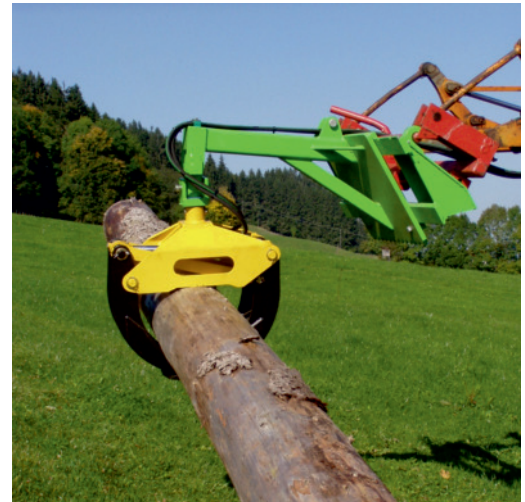
equipped with mechanical rotation linkage
