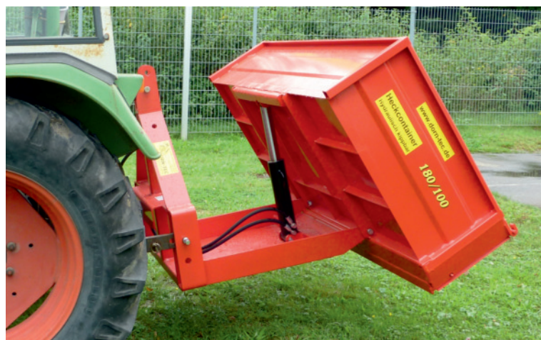
equipment with extra strong hydraulic cylinder - single or double acting
