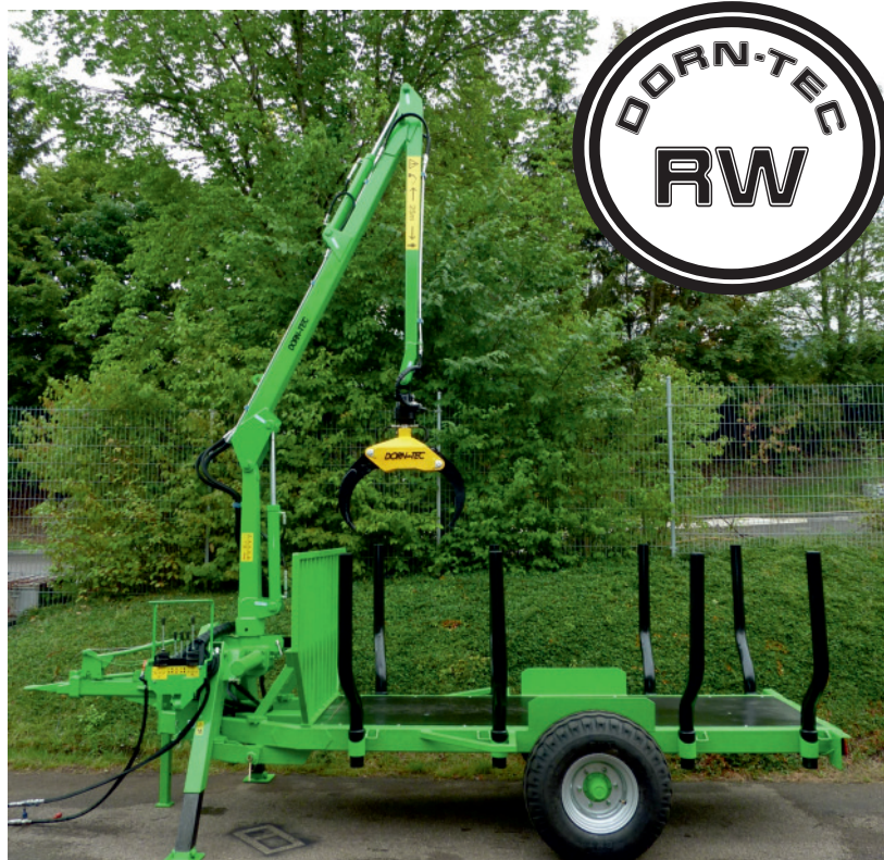
single-axle firewood trailer RW60 [6,0to] with crane KCF3 - reach 4,8 m
