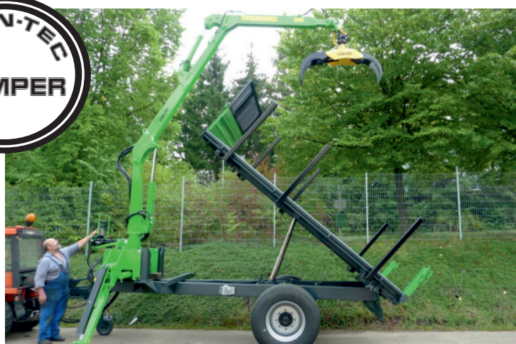
tilt-platform with optional construction for stakes
