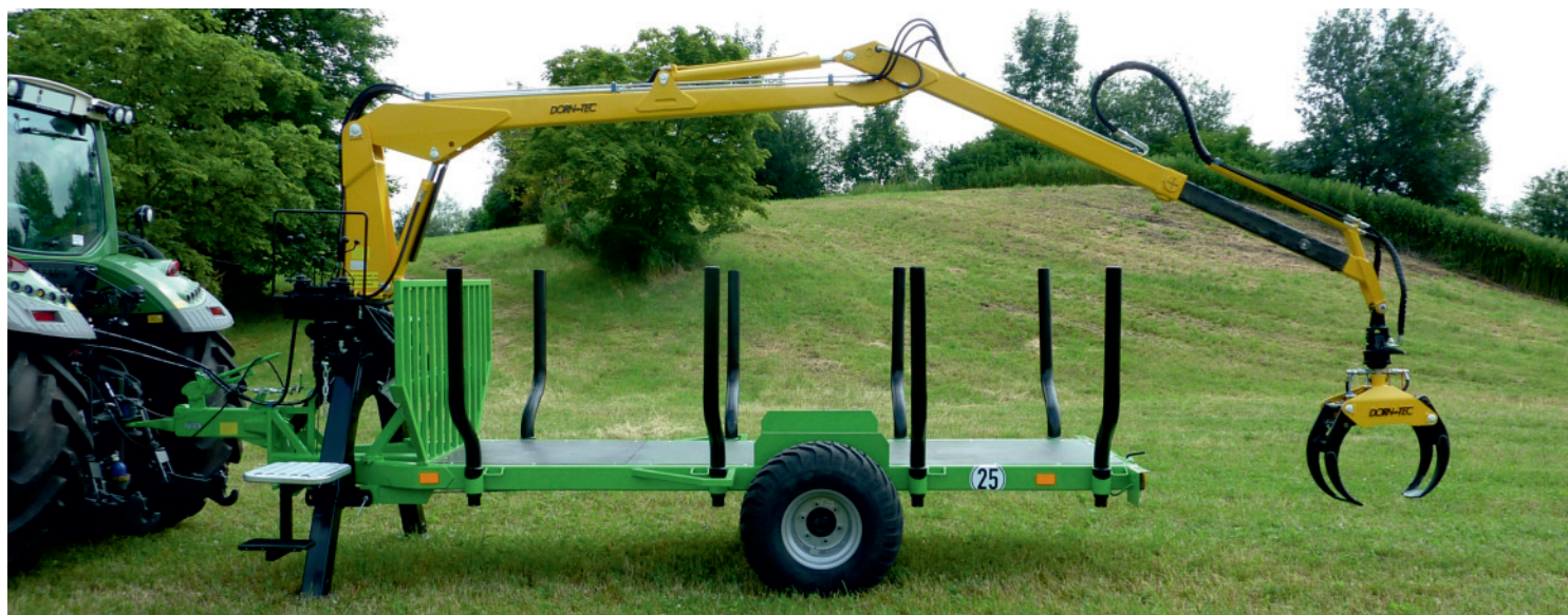
single-axle forestry trailer Rw80 [8,0to.] with crane 650 - telescopic arm and max. reach 6,9 m
