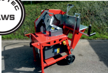
circular saws with swinging table
