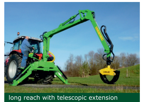
three-point attachment with seat on column
