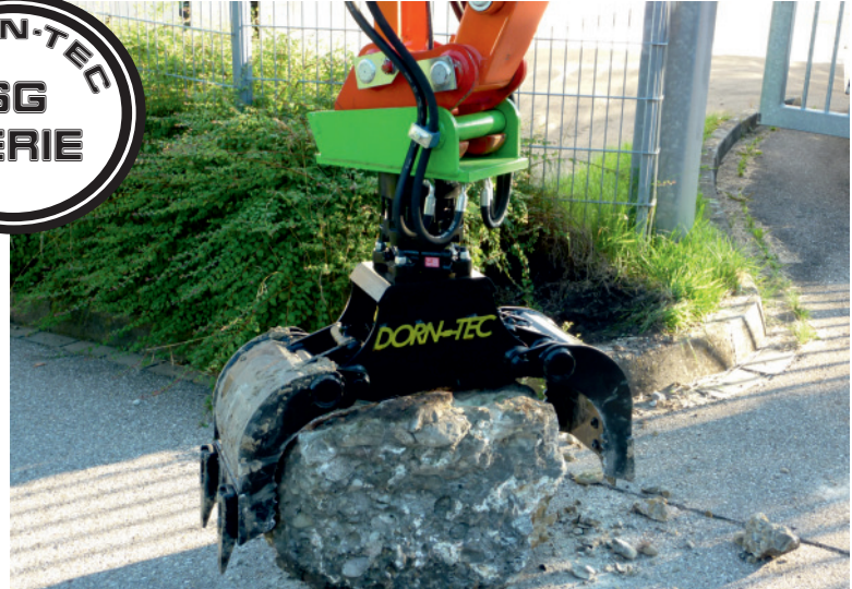
Stone grab with quick-coupler connection and closed peelings
