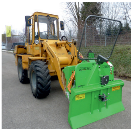
winch with hydraulic drive
