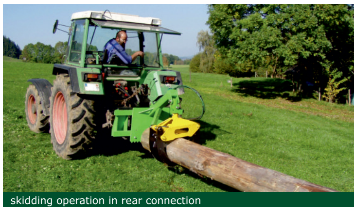
high rear lifting with integrated three-point
