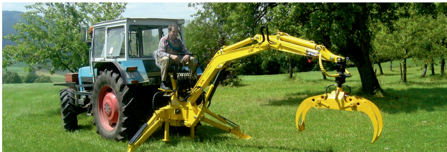
combi backhoe loader for digging and loading with revolving hydraulic flap-down stabilizers, seat on column and EURO-control valve
