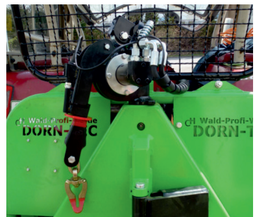
pulley with hydraulic drive & stop-switch
