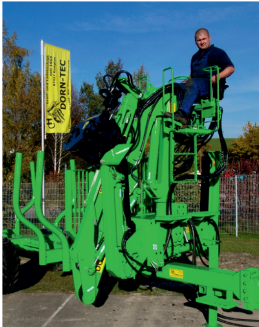
Z-crane with comfort control and seat
