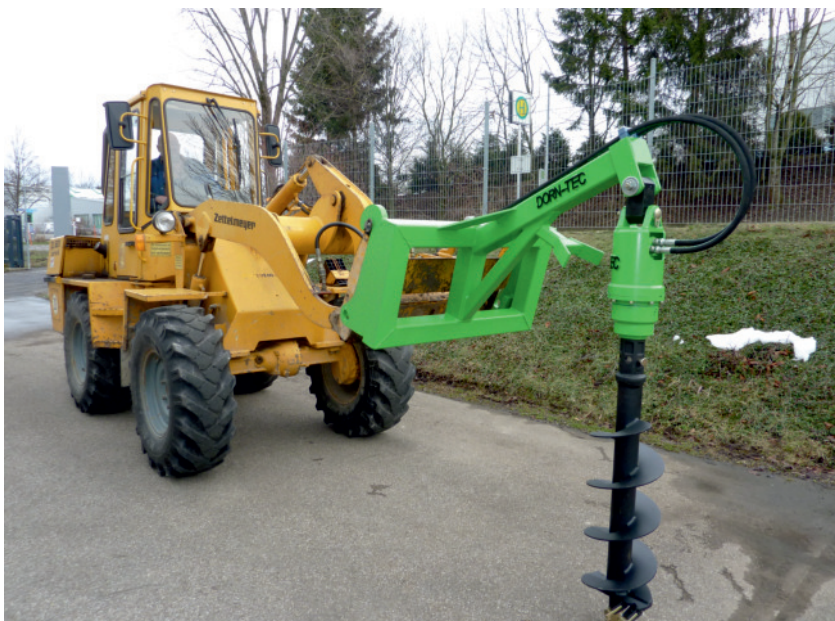
adaptation made by DORN-TEC - augers in use on a front or wheel loader
