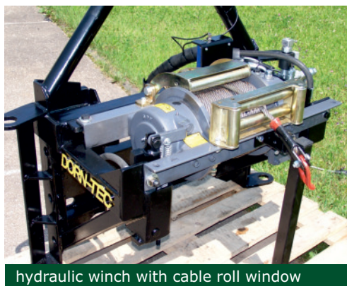
compact winches with planetary gear units for lifting equipment
